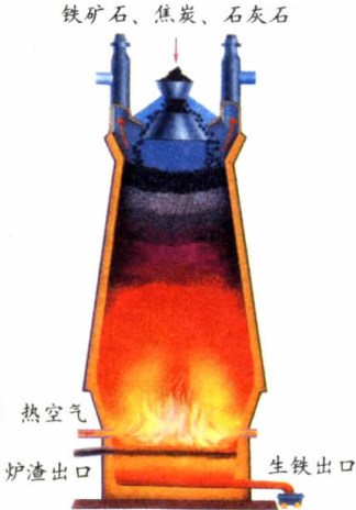
图 5 炼铁高炉及炉内化学变化过程示意图 Fig. 5 Schematic diagram of ironmaking blast furnace and chemical reaction process in furnace
