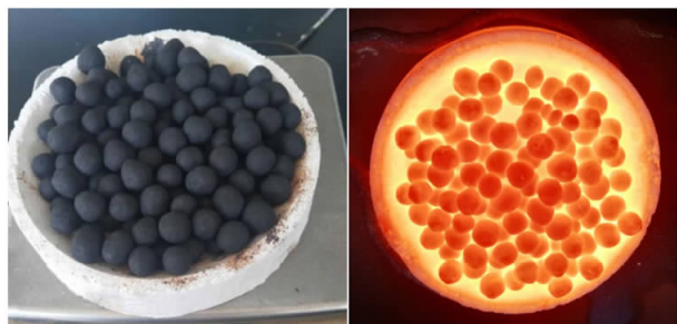
图5 球团焙烧前(左图)与焙烧后(右图)形貌 Fig. 5 Appearance of pellets before (left) and after (right) roasting
