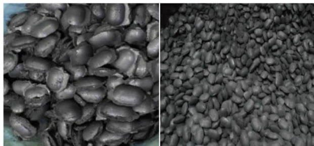
图4 湿球(左)与干球(右)形貌 Fig. 4 Image of wet pellets (left) and dry pellets (right)
