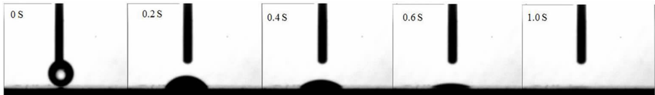
图 4 强亲水电极材料表面的连续动态接触角测量图像 Fig. 4 Images of continuous dynamic contact angle for strong hydrophilic electrode material
