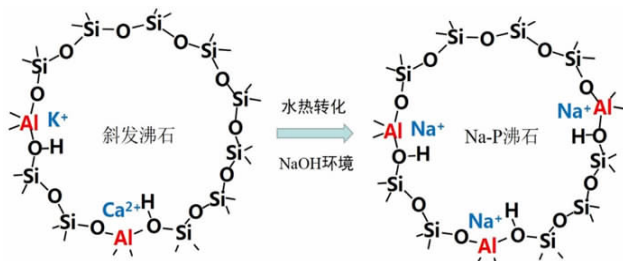
图 9 斜发沸石和水热转化 Na - P 沸石的结构示意图 Fig. 9 Structure schematics of clinoptilolite and hydrothermal transferred zeolite Na - P
