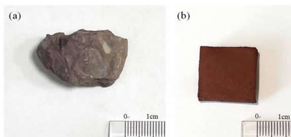
图 1 清水泥矿料(a)、泥坯(b)照片 Fig. 1 The photographs of (a) Qingshui Zisha clay mineral, and (b) wet green body of Qingshui clay of Qingshui Zisha
