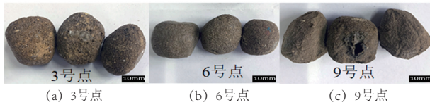
图2 不同粒径铁尾矿陶粒照片 Fig. 2 Photos of ceramsites using iron tailings with different particle sizes
