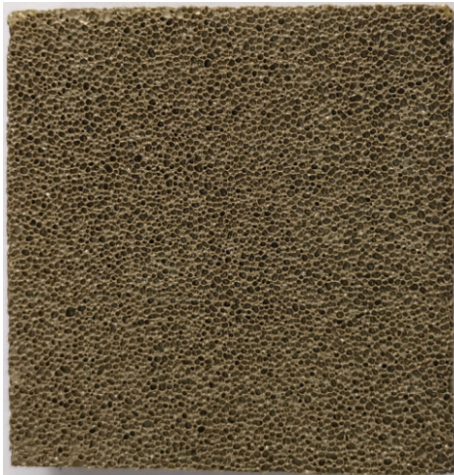
图5 磁选后石墨尾矿制备的发泡陶瓷样品 Fig. 5 Foamed ceramic samples prepared from graphite tailings after magnetic separation
