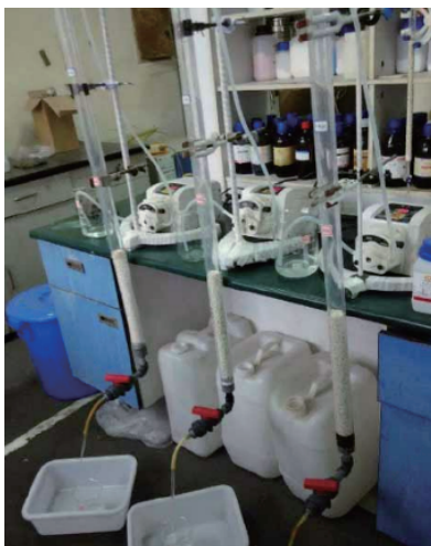
图 9 动态循环吸附装置及循环工艺流程 [96] Fig. 9 Dynamic cyclic adsorption device and cyclic process flow chart [96]
